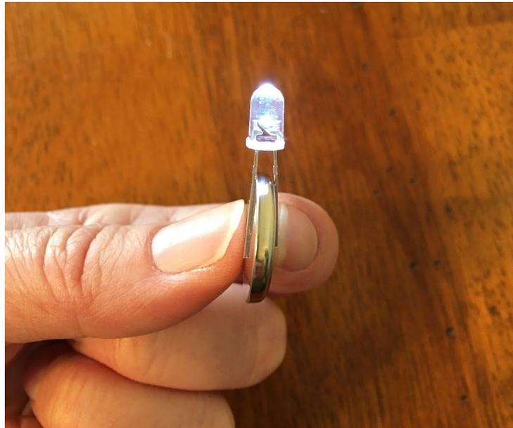
13. Once the light is lit, hold the prongs in place by wrapping the electrical tape around the prongs and battery.
